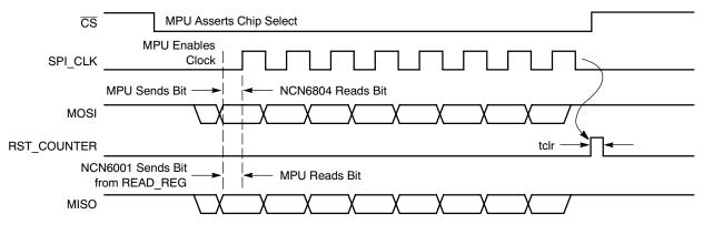
Figure 11. Basic SPI Timings and Protocol
