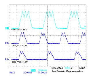
**Figure 19. Typical Inductor Current**
