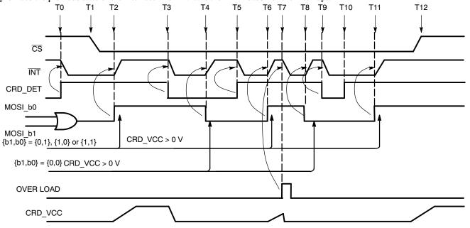
Figure 10. Basic Interrupt Function
