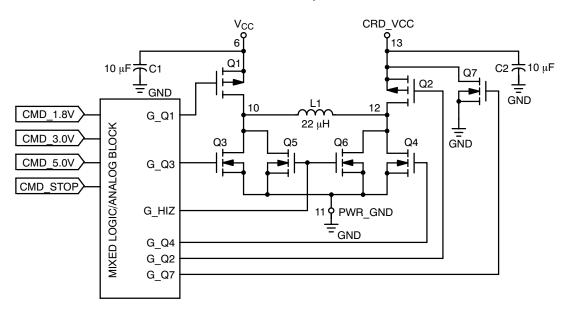
Figure 16. Basic DC/DC Converter
