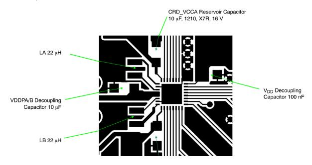
Figure 25. Example of PCB Device Implementation
