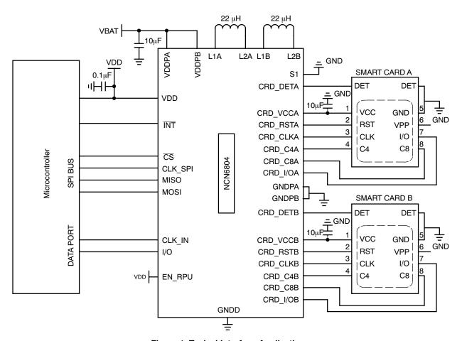
Figure 1. Typical Interface Application
