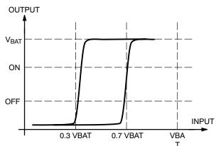
Figure 24. Typical Schmitt Trigger Characteristic
