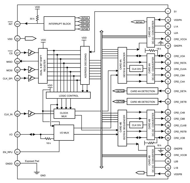
Figure 2. NCN6804 Block Diagram
