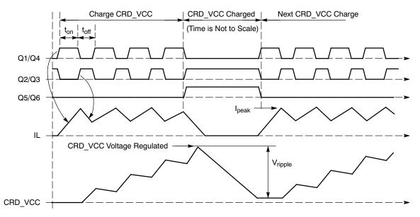
Figure 17. Theoretical DC/DC Operating Waveforms
