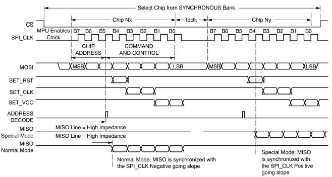
Figure 13. Basic Multi Command SPI Bytes
