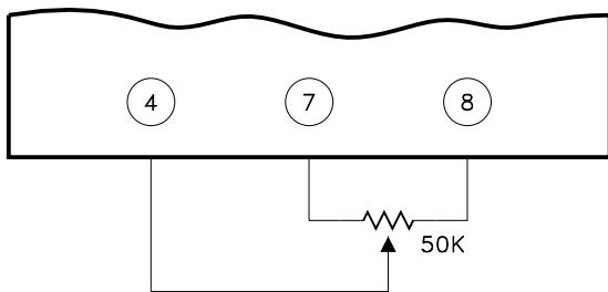
Adjust/comp (pin 4) may be driven by external circuitry referenced to pin 8 (-output sense) if desired. Grounding pin 4 causes output voltage to increase (25% typically) while driving pin 4 above 1.3V causes output voltage to decrease. Pin 4 may be driven through 10KΩ or more if connection of the comp function is also required.
