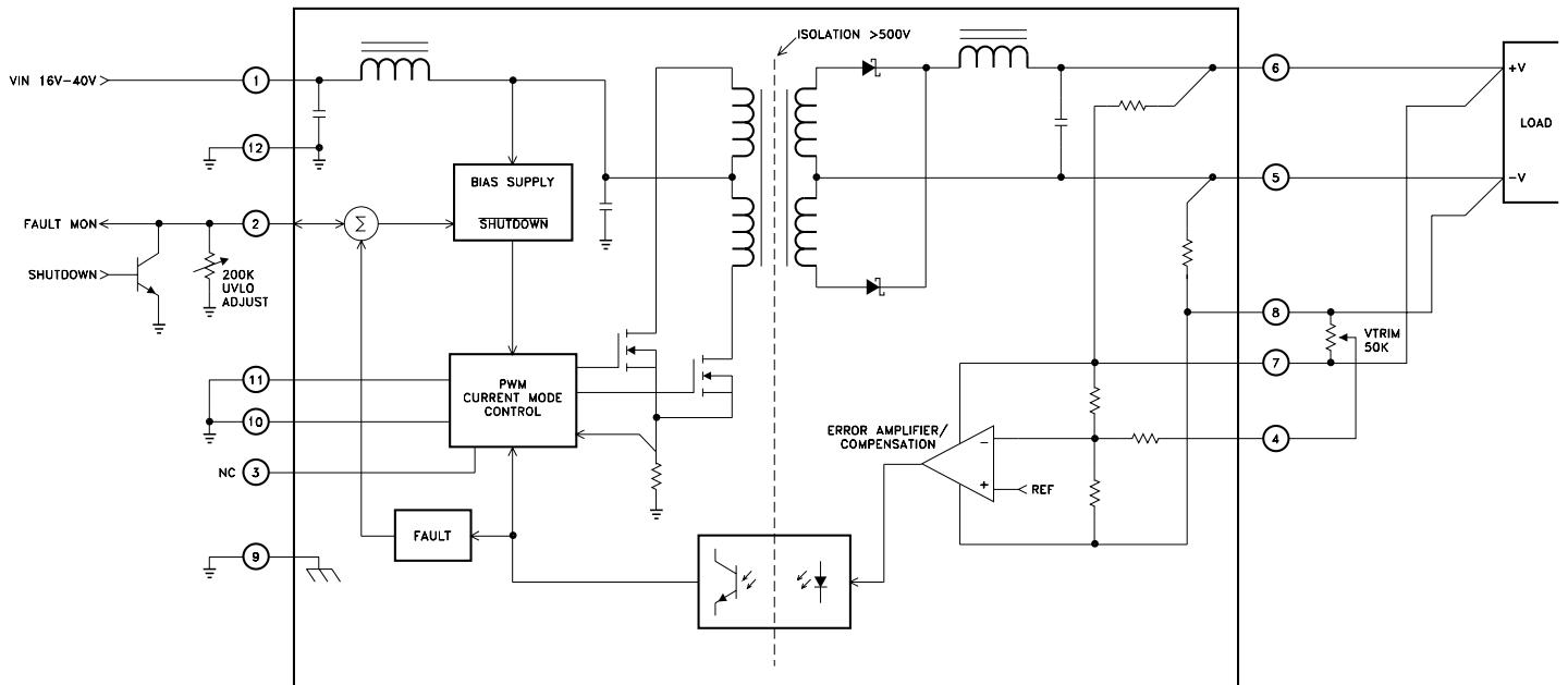
The above diagram shows the remote sense feature which reduces  $V_o$  errors due to the resistance of the conductors feeding the load. This diagram also shows the connections for non-synchronized operation (TIMING 1 and 2) as well as output voltage trim, remote shutdown, fault monitoring, and input voltage turn on point adjustment.
