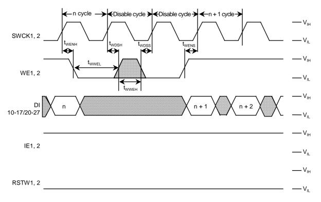
Write Cycle Timing (Write Enable): MODE1 =  $V_{ss}$
