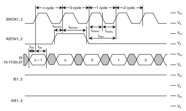
Write Cycle Timing (Write Reset): MODE1 =  $V_{CC}$
