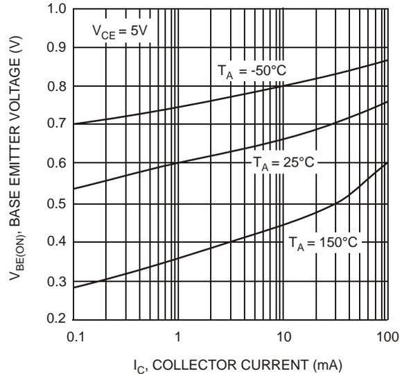
Fig. 4, Base Emitter Voltage vs. Collector Current
