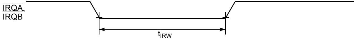
Figure 10-6 External Interrupt Timing (Negative Edge-Sensitive)
