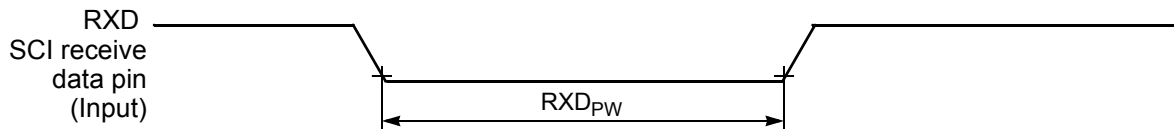
Figure 10-15 RXD Pulse Width
