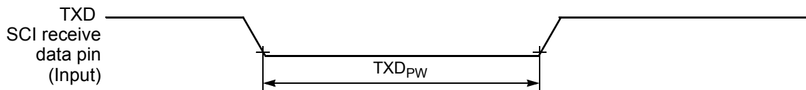
Figure 10-16 TXD Pulse Width
