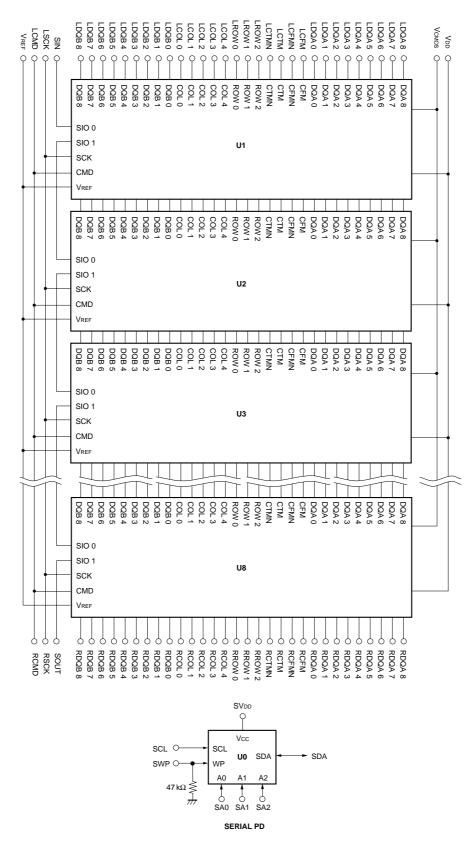
**Remarks 1.** Rambus Channel signals form a loop through the SO-RIMM module, with the exception of the SIO chain.
