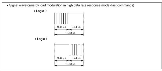
Data frame: A data frame sent from a transponder starts with a start-of-frame (SOF) signal and ends with an
