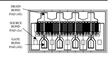
DIE SIZE: 28.3X16.5 mils (720x420 µm) DIE THICKNESS: 2.6 mils (65 µm) BONDING PADS: 1.9X2.4 mils (50x60 µm)
