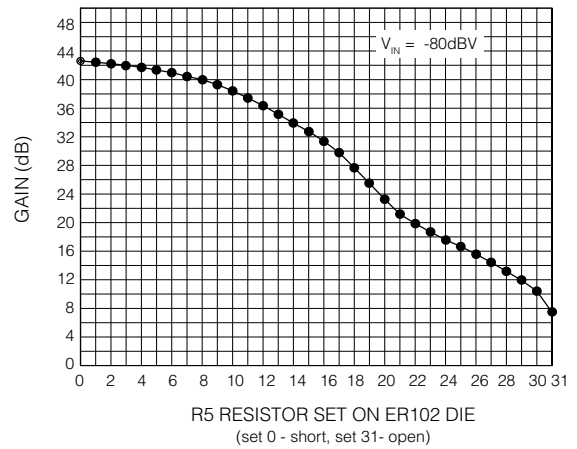
Fig. 6 High Frequency Gain (Compression Ratio Adjustment)
