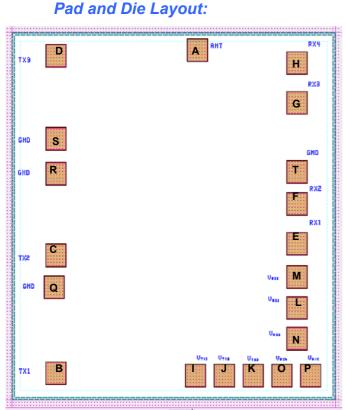
**Note:** Co-ordinates are referenced from the bottom left hand corner of the die to the centre of the bond pad opening
