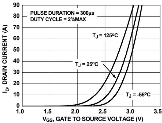
Figure 5. Transfer Characteristics
