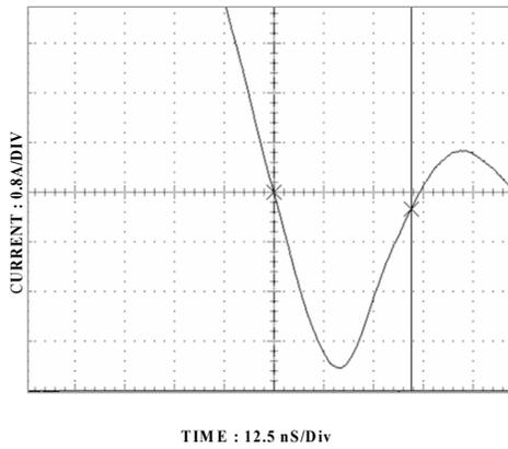
Figure 14. FDMS8660S SyncFET body diode reverse recovery characteristic
