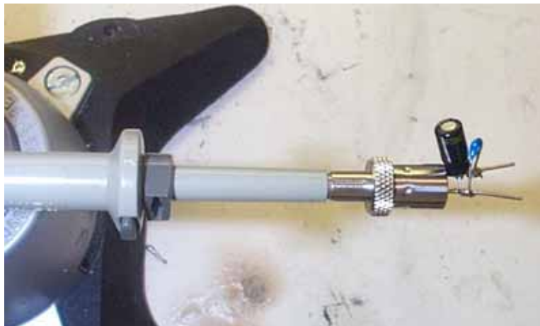
Figure 31 – Oscilloscope Probe with Probe Master 5125BA BNC Adapter (Modified with Wires for Probe Ground for Ripple Measurement, and Two Parallel Decoupling Capacitors Added).
