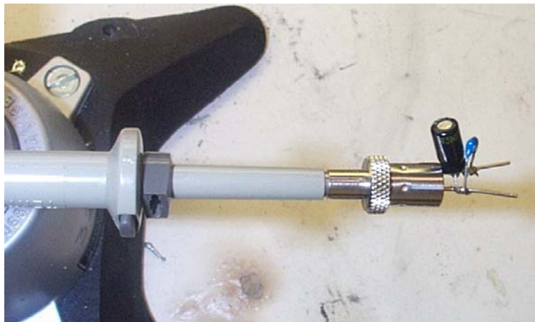
Figure 10 – Oscilloscope Probe with Probe Master 5125BA BNC Adapter
