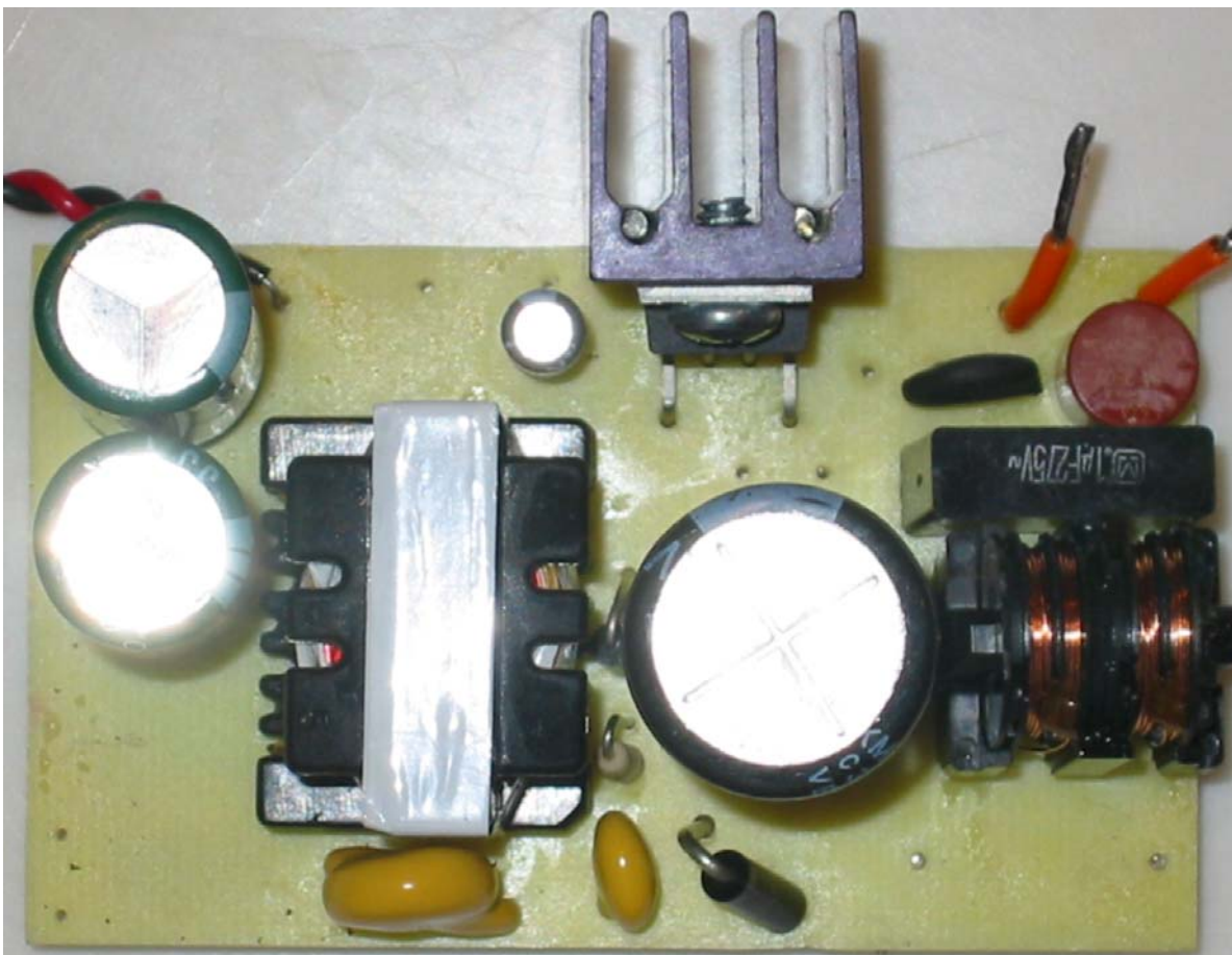
Figure 1 – Power Supply Prototype – Top View
