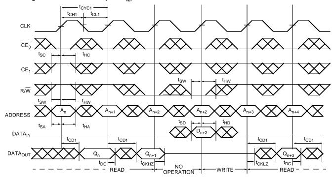
Flow-Through Read-to-Write-to-Read (OE Controlled)[12, 14, 21, 22]
