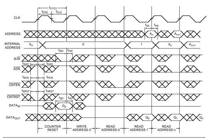
Notes: 27.  $\overline{CE}_0$ ,  $\overline{UB}$ , and  $\overline{LB} = V_{IL}$ ;  $CE_1 = V_{IH}$ .
