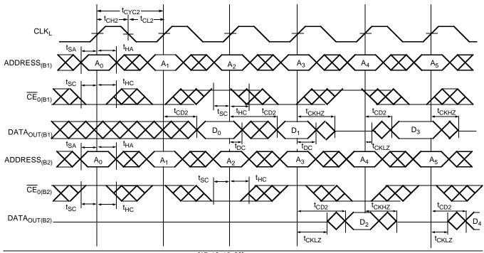
Left Port Write to Flow-Through Right Port Read<sup>[17, 18, 19, 20]</sup>
