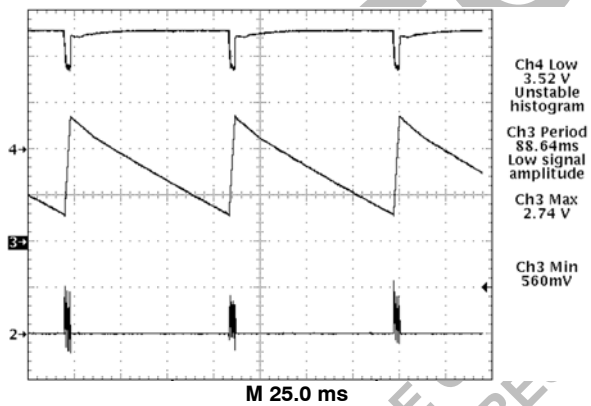
Figure 12. CS5158 Demonstration Board Hiccup Mode Short Circuit Protection. Gate Pulses are Delivered While the Soft Start Capacitor Charges, and Cease During Discharge
