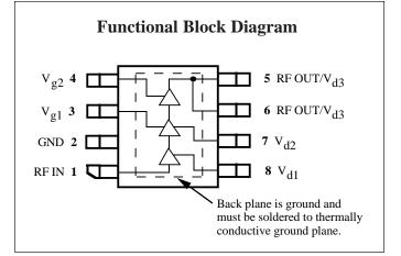
and flexibility. The CMM0330 is packaged in a low-cost, space efficient SO-8 power package that gives excellent electrical stability and thermal handling performance with a  $R_{\Theta}$  of less than 18° C/W. The part is designed to require minimal external circuitry for bias matching, simplifying design and keeping board space and cost to a minimum.
