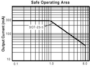
Input-Output Voltage Differential (V)
