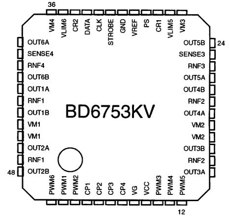
Fig.2 BD6753KV Pin Arrangement (Top View)
