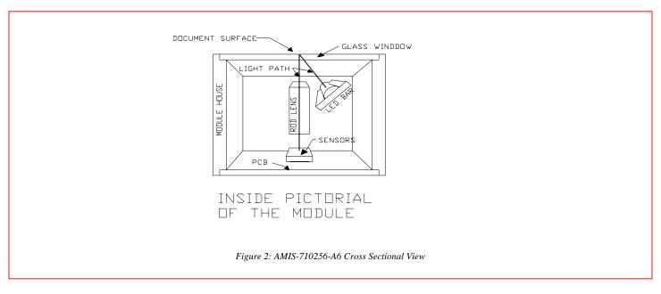
This pictorial cross section shows the LED bar light source and its illumination path. The light on the document reflects images of the document. The reflected images focus through the micro lens onto the image sensing line of the chips, where images are converted to proportional electrical charges. An on-board amplifier processes these signal charges into proportional video signal voltages, which are sent out to the output video port.
