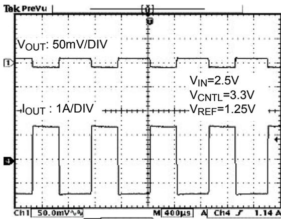
Fig. 8 Transient Response at 1.25V<sub>TT</sub>/1.5A
