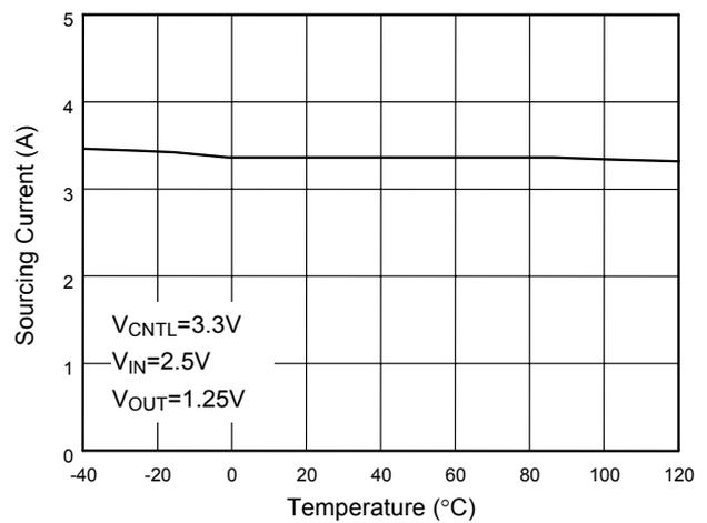
Fig. 4 Current-Limit (Sourcing) vs. Temperature
