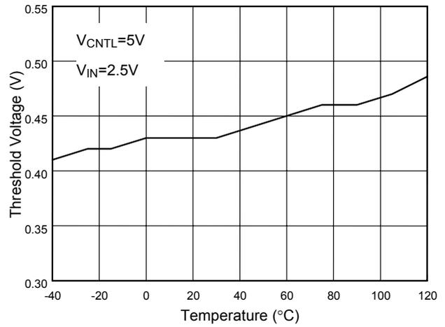
Fig. 2 Turn-On Threshold vs. Temp
