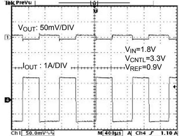
Fig. 9 Transient Response at 0.9V<sub>TT</sub>/1.5A
