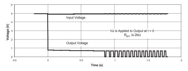
Figure 1: Overload Operation.
