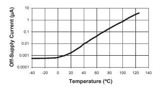
Off-Switch Current vs. Temperature
