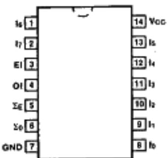
**DESCRIPTION** — The '180 is a monolithic, 8-bit parity checker/generator which features control inputs and even/odd outputs to enhance operation in either odd or even parity applications. Cascading these circuits allows unlimited word length expansion. Typical application would be to generate and check parity on data being transmitted from one register to another. Typical power dissipation is 170 mW.
