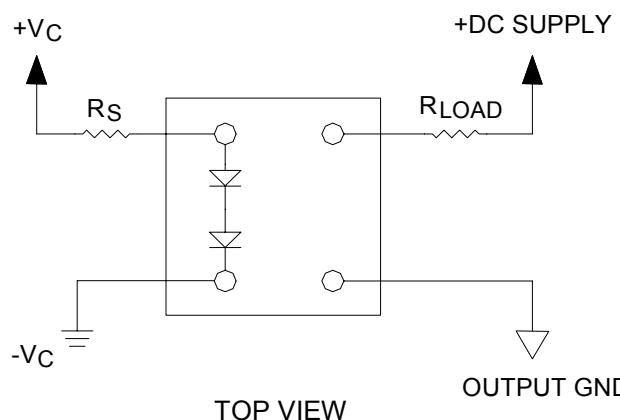
Figure 2. Terminal Connections
