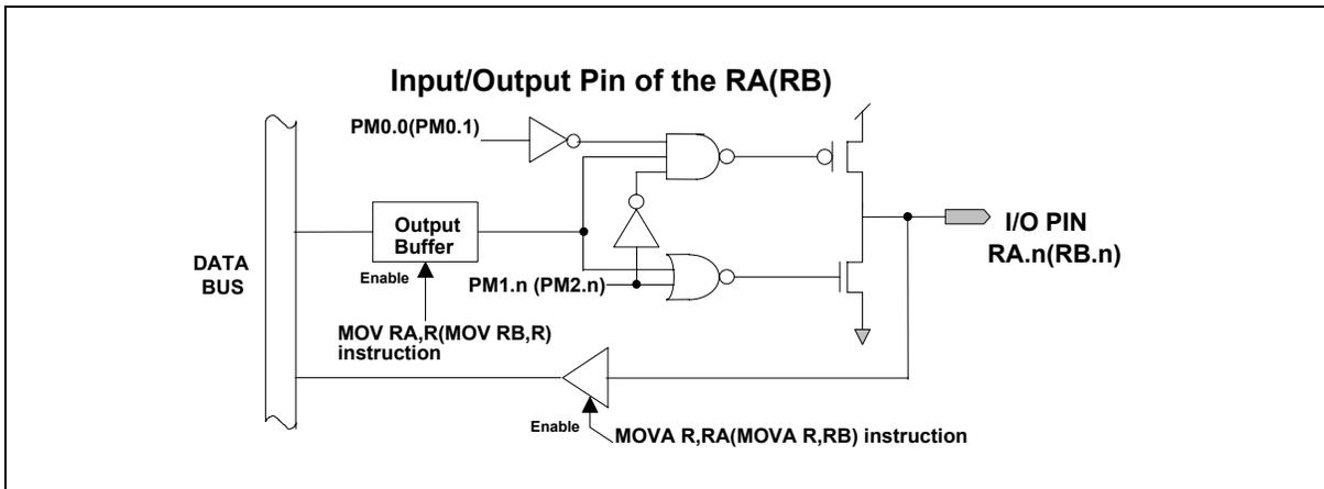
Figure 6-11 Architecture of RA (RB) Input/Output Pins
