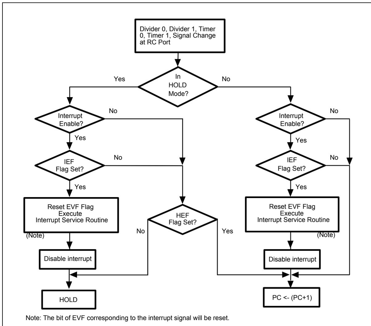
Figure 6-9 Hold Mode and Interrupt Operation Flow Chart
