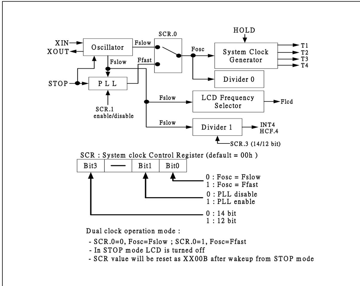
Figure 6-4 Organization of the dual-clock operation mode
