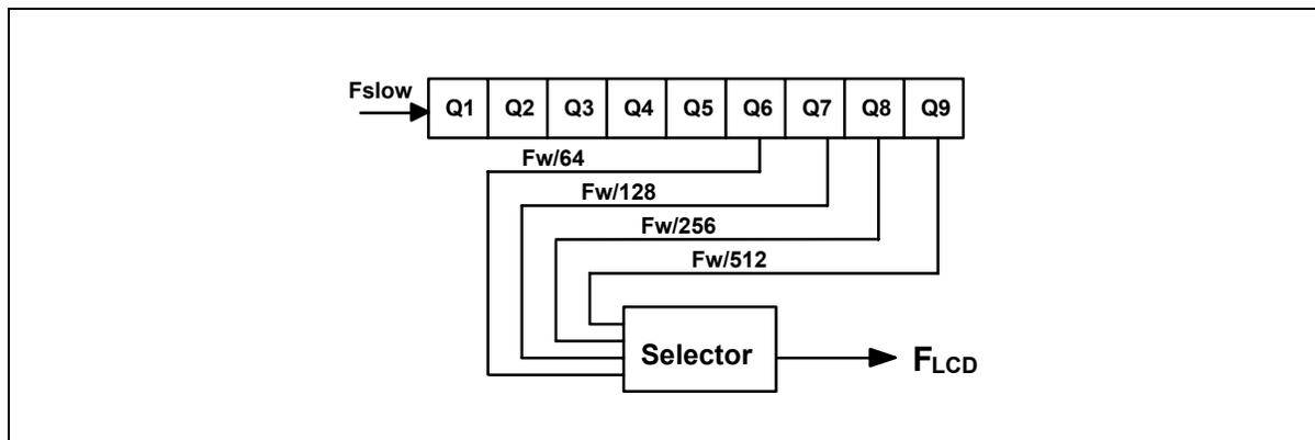
Figure 6-15 LCD alternating frequency (FLCD) circuit diagram
