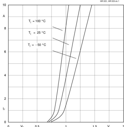
Fig. 1 Forward characteristic ( typical values )
