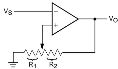
$$V_{UL} = \{R_1/(R_1 + R_2)\} V_O(max)$$
