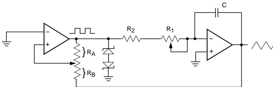
$$\text{frequency} \propto R_1, R_2, C$$
