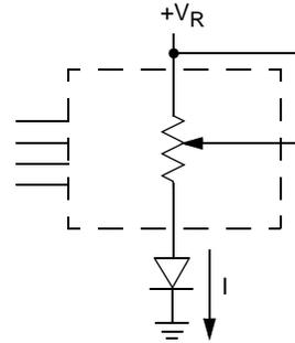
Two terminal Variable Resistor;
