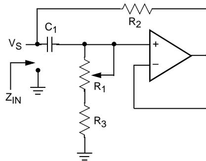
$$Z_{IN} = R_2 + s R_2 (R_1 + R_3) C_1 = R_2 + s L_{eq}$$
