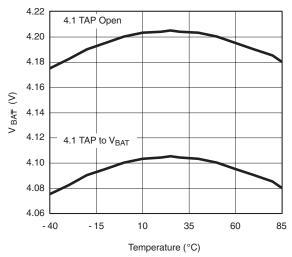
V<sub>BAT</sub> (CV Mode) vs. Temperature
