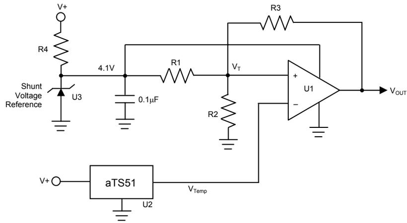
**Figure 6. Thermostat/Fan Controller**
