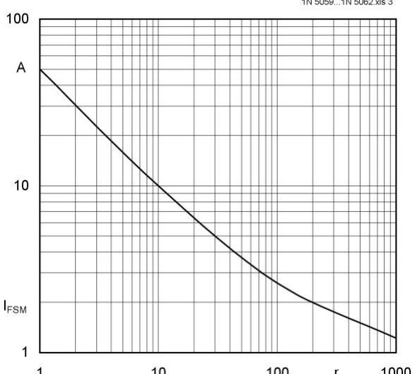
Fig. 3  $I_{FSM}$  current versus number of cycles at 50 Hz
