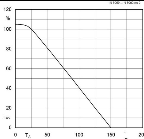
Fig. 2 Rated forward current vs. ambient temperature <sup>1)</sup>
