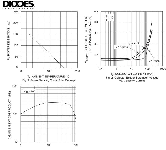
I<sub>C</sub>, COLLECTOR CURRENT (mA) Fig. 3, Gain Bandwidth Product vs Collector Current
