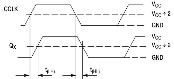
Figure 8. Propagation delay ( $t_{pD}$ ) test reference
