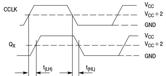
$$t_{SK(P)} = |t_{PLH} - t_{PHL}|$$
