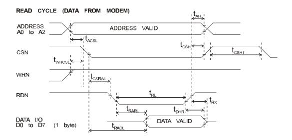
Figure 5 µController Parallel Interface Timings
