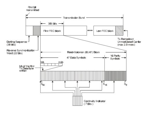
Figure 3 Reverse Channel Transmission Structure
