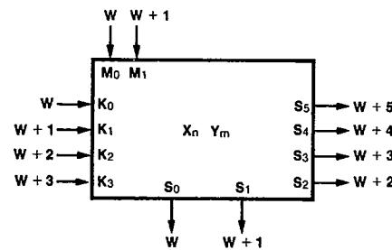
This block represents the basic 4-bit by 2-bit multiplier, and indicates the weighting factors (power of two) attached to each of the inputs and outputs.
