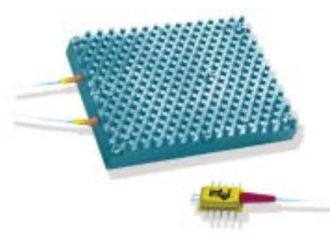
The TXN13210/11/14 transceiver family can be configured to supply a single- or dual-rate SONET/SDH or 10Gb Ethernet interface, with clock jitter filtering. The module satisfies link distances from 0 to 10km. Various heat sink and optical connector options are available to satisfy a range of applications. The transceiver is assembled in a Multi-Source Agreement (MSA)-compatible package that is a minimum size of 3.0" L x 2.2" W x 0.43" H.
