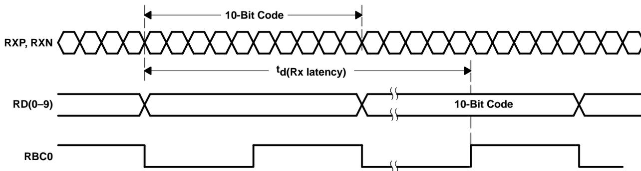
Figure 6. Receiver Latency – TBI Normal Mode Shown
