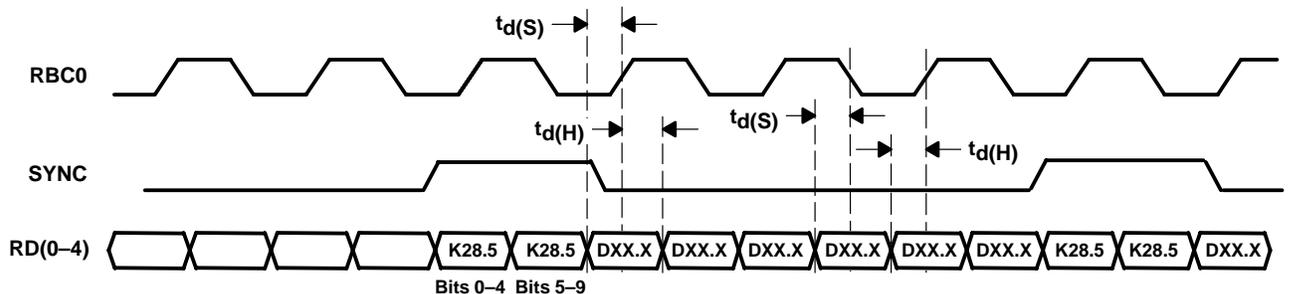
Figure 4. Synchronous Timing Characteristics Waveforms (DDR mode)
