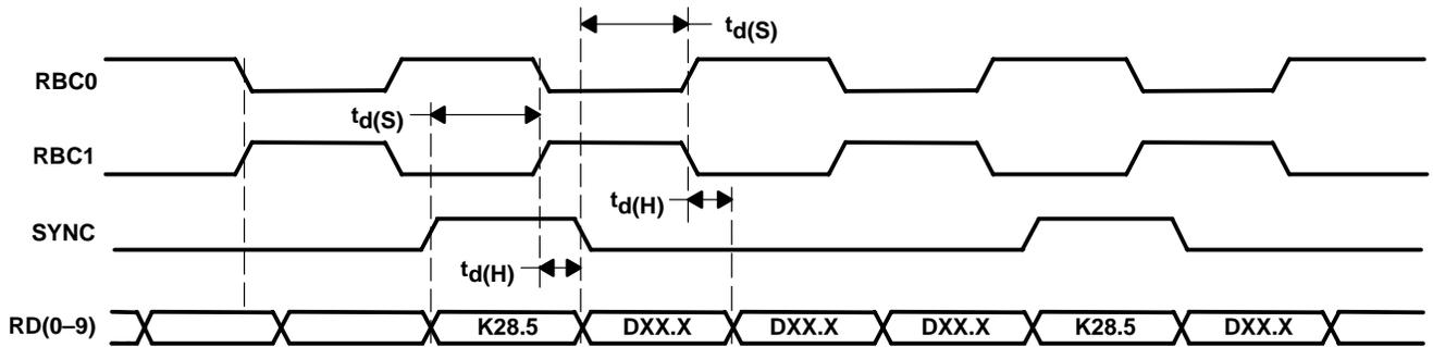
Figure 2. Synchronous Timing Characteristics Waveforms (TBI half-rate mode)
