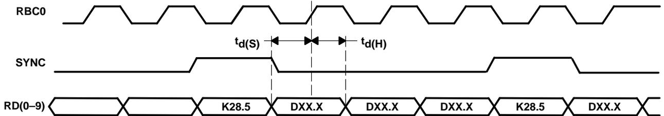
Figure 3. Synchronous Timing Characteristics Waveforms (TBI full-rate mode)
