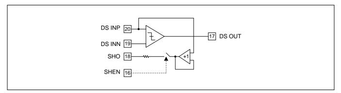
The output of the data slicer (DS-OUT) is a CMOS compatible bitstream. However, it is recommended that an external NPN amplifier stage be used to drive the CMOS baseband processor, in order to minimize the amount of ground and supply currents in the S1T8536 which might desensitize the chip.
