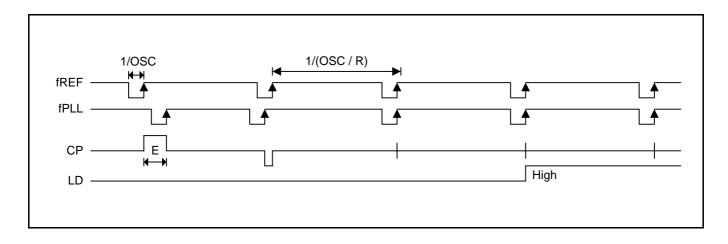
When the situation that E(error) is less than one period of reference frequency, 1/OSC, continues more than three cycles of reference counter output, 1/(OSC/R), lock detector outputs 'High'.
