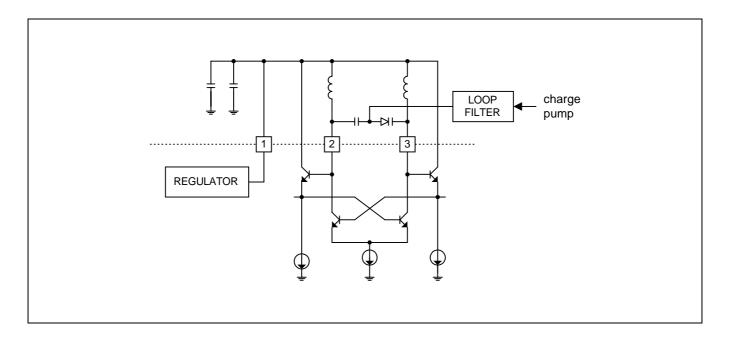
Following figure shows external components in case of using external VCO.
