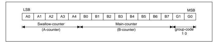
5-Bit Swallow Counter (A-Counter) Division Ratio A =  $A4*2^4 + A3*2^3 + A2*2^2 + A1*2^1 + A0*2^0$ Division ratio : 0 to 31, A < B
