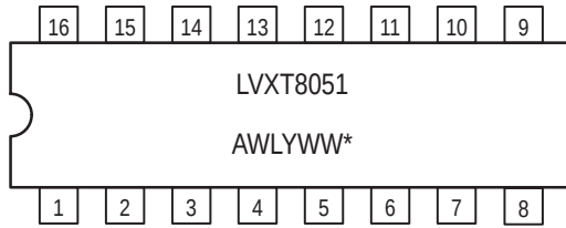
16-LEAD SOIC D SUFFIX CASE 751B
