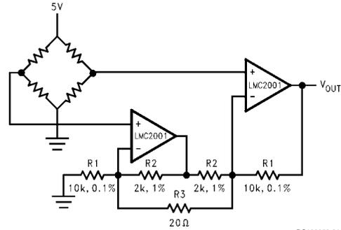
**FIGURE 4. Single Supply Strain- Gauge Amplifier**
