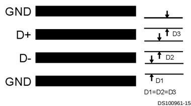
FIGURE 6. Recommended Diode Trace Layout
