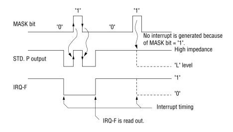
Periodic timing waveform output mode (INT/STND = "0")
