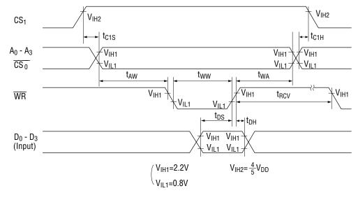
The ML9070-03 has no  $\overline{\text{CS}}_0$  input. (Note)
