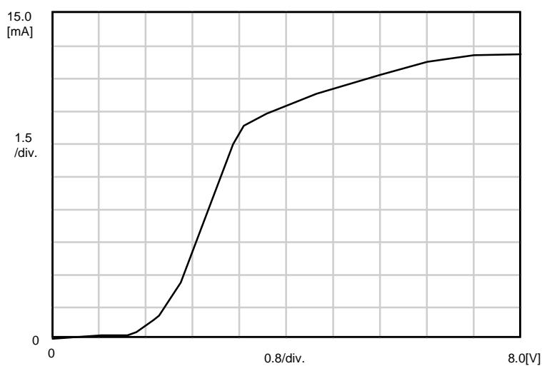
**1.  $V_{CC}$  vs.  $I_{CC}$** **V<sub>ref</sub>**
