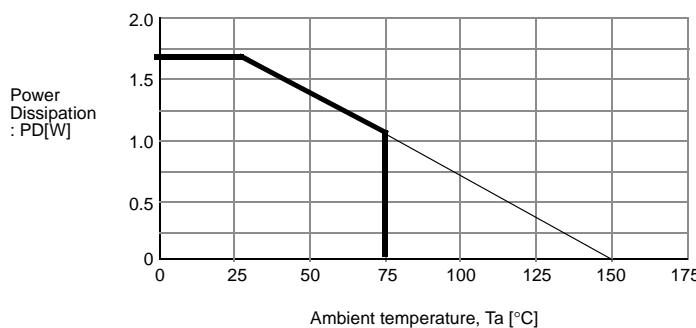
Power dissipation decreases in the rate of 13.5mV / °C when mounted on 50mm × 50mm × 1mm PCB (Phenolic resin material) and used above Ta=25°C.
