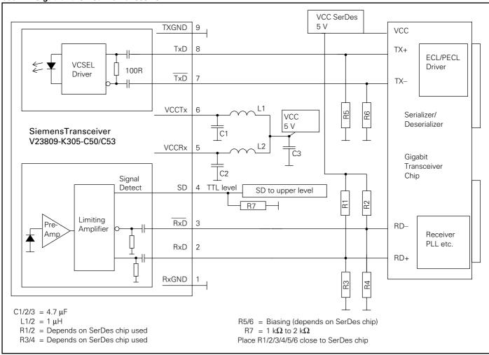
Values of R1/2/3/4 may vary as long as proper  $50\,\Omega$  termination to V<sub>EE</sub> or 100  $\Omega$  differential is provided. The power supply filtering is required for good EMI performance. Use short tracks from the inductor L1/L2 to the module V<sub>CC</sub>RX/V<sub>CC</sub>TX.
