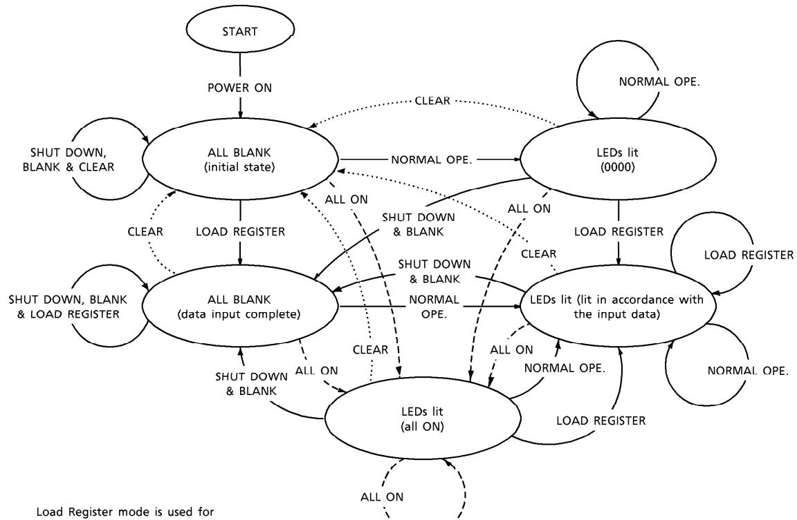
Load Register mode is used for the detail settings for the digit output duty cycle, for setting Decode/No Decode, for inputting display data, and for setting the number of digits to use.
