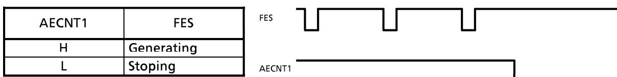
AECNT1 is not allowed to change while FES pulse is "L" level. Because AECNT1 gates FES pulse.
