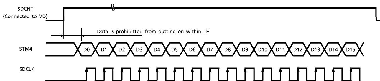
SDCNT is connected to VD of synchronization generator IC.
