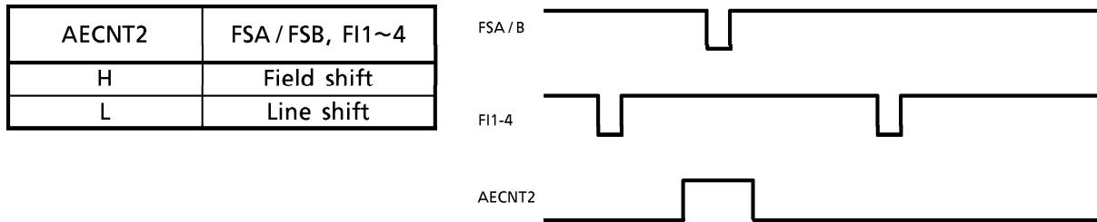
The period of "H" level on AECNT2 should be longer than the holding period of "H" level as follows. AECNT2 is not allowed to change 9H before FSA / B and 10H after FSA / B.
