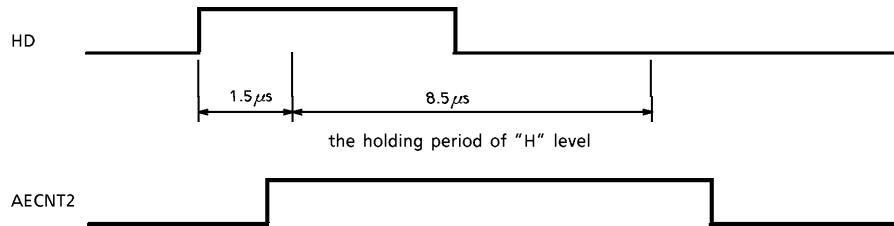
On AECNT mode, generation of trigger pulse needs external counter circuits. And VTG pulse is used for the standard pulse resetting the external counter circuits. The time difference of VTG and field shift(shutter OFF) in the next field are set as follows;
