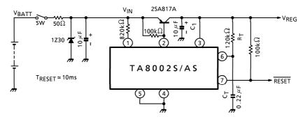
2. Application Circuit Using Darlington Transistor
