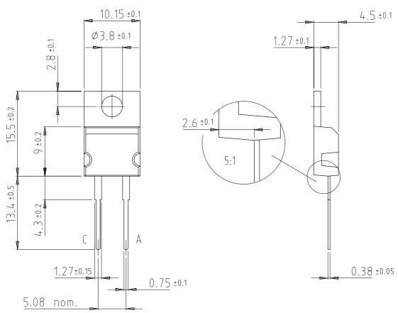
Plastic case JEDEC DO 220 Cathode connected with metallic surface technical drawings according to DIN specifications
