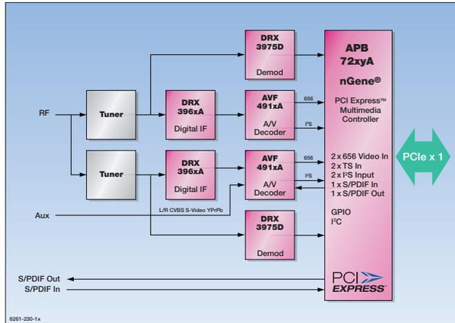
Fig. 2: Dual-channel TV tuner with PCI Express™
