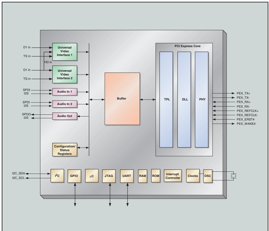
Fig. 3: Block diagram of the APB 7202A
