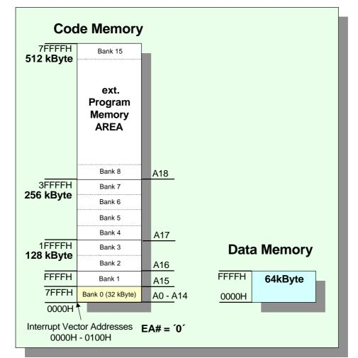
The following figure gives an overview of the 'Expanded Configuration'.
