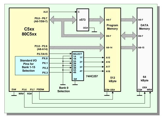
Figure 3: Schematic for External Memory Bus Interface
