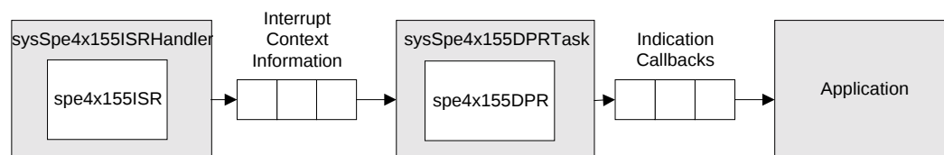
Figure 6: Interrupt Service Model
